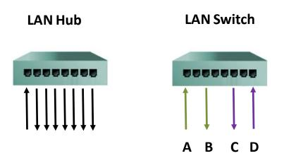
Figure 3. LAN Hub and Switch
