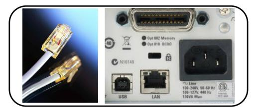
Figure 1. LAN Cable and RJ45 Connection
